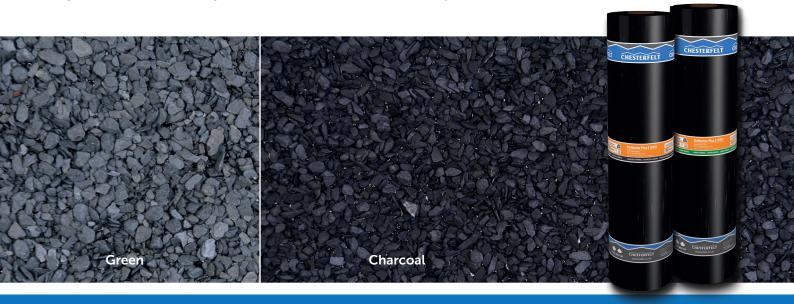
Deflector Plus 5 cap sheets are designed for use on various types of flat roofing projects including new build and refurbishments, cold roofs and warm roofs using vapour control layers with insulation. They feature a polyester core which is saturated and coated in SBS modified bitumen and the upper surface is finished with a choice of green or charcoal slate mineral.
