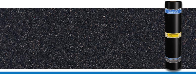
Chesterfelt Laser Gold Underlay features a glass fibre core and is designed to be used as part of a torch-applied built-up roofing system. It incorporates SBS modified bitumen and has a light sanded finish on the upper surface. Waterproofing is achieved by saturating and coating both surfaces in bitumen.
